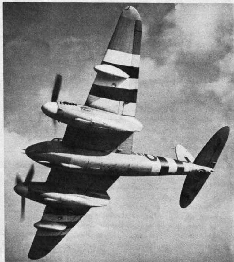
Mosquito in plan has graceful curves, is one of the cleanest airplanes. Radiators on leading edge of wing appear on both Hornet and Mosquito.
